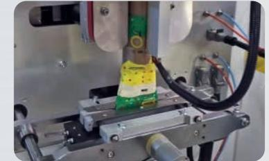
**Auger filler:** A simple design for small pouches with high capacity is possible with our Mini vertical form fill and seal machines. Up to 17 cm bag width and 25 cm bag, length flexibility covers mostly needed packaging demands as well as to fill 1 kg of granule products maximum.
